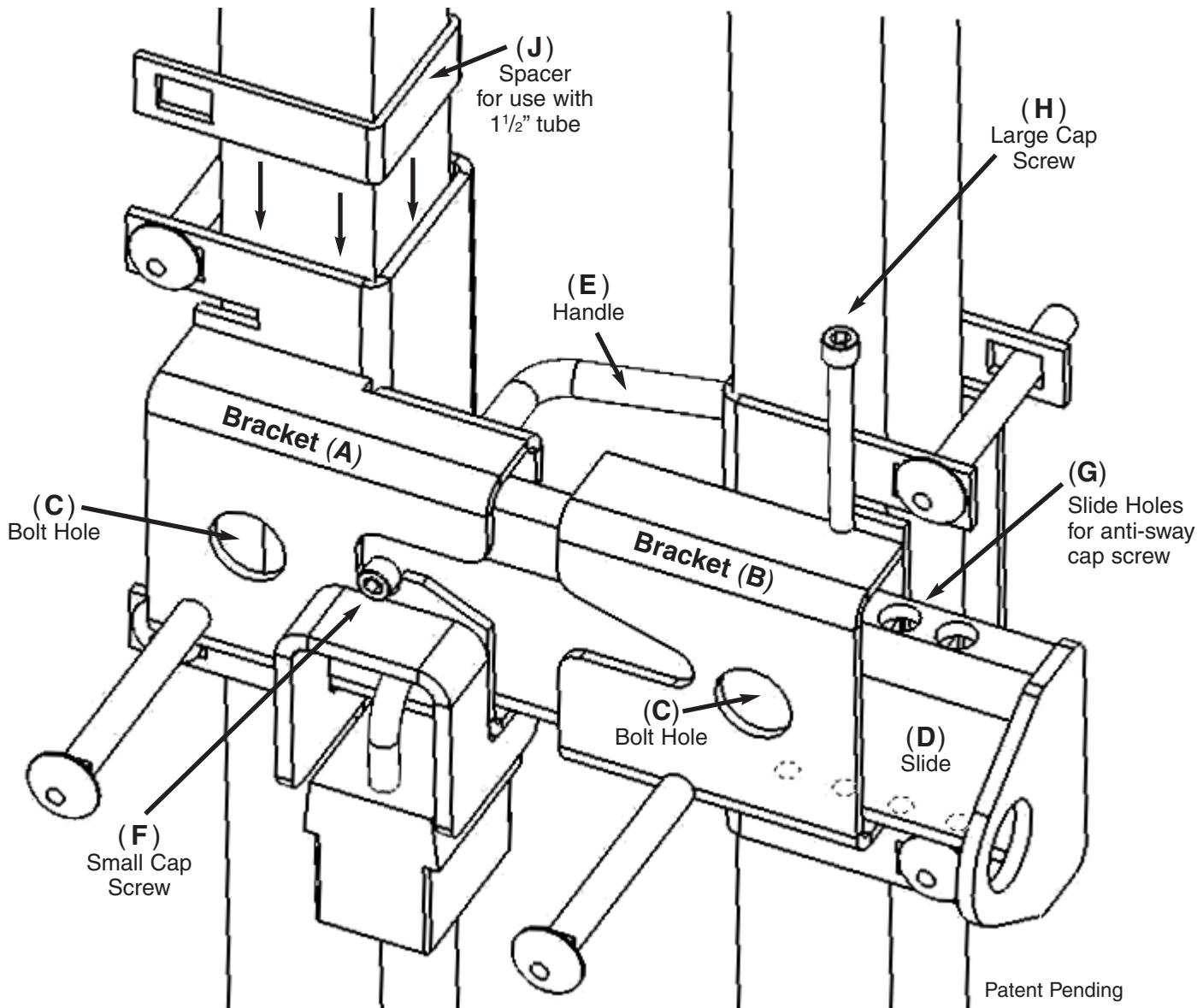
1. Attach latch to Gate Frames. Make sure Brackets (A & B) are aligned and level before tightening bolts.
