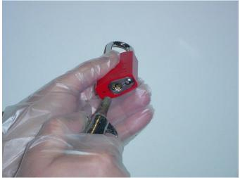
• In particularly filthy areas it may be necessary to also flush dirt and grease from the padlock with WD-40 or Brake Parts Cleaner. When clean, the ball bearing you can see inside the shackle hole should move back and forth easily.
