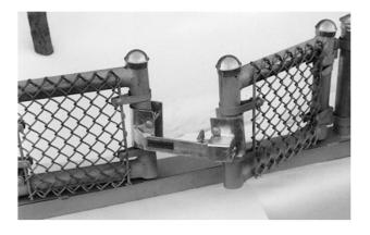
Rotating enables each latch piece to slide into one another at the correct alignment.
