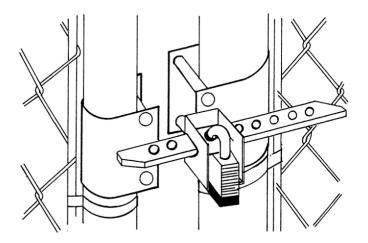
When gates are in a closed position, latch can now be padlocked through aligned holes.
