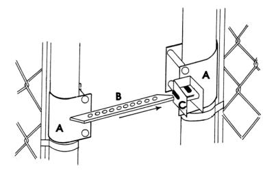
Install Brackets A so they rotate and enable Bar B to line up with C.
