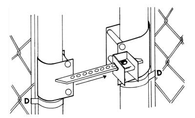
• Use Tension Bands **D** to keep latch in proper alignment adjustment.
